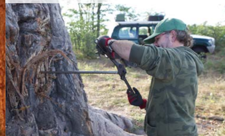
Dr Grant, extracting a Baobab core sample for analysis in the Stable Isotope Laboratory at UP
